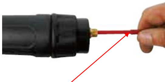
(3) Carefully pull out and completely remove the liner.
