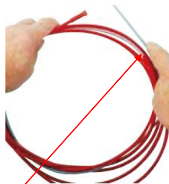
(4) Carefully unravel the new liner
